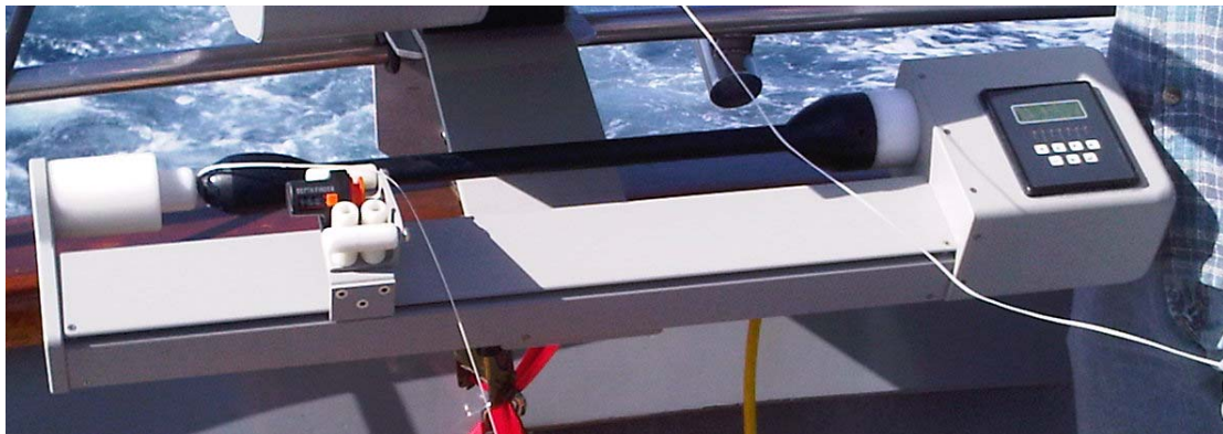
Figure 2 UnderwaySV rewinder with tail spool loaded for rewinding.
