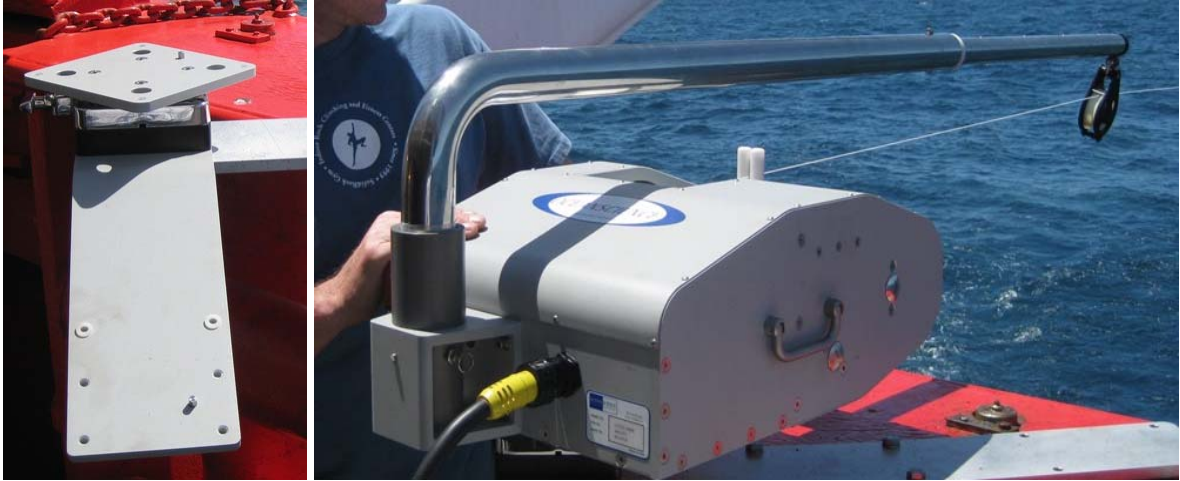
Figure 3 Rewinder and winch mounts (left) on the gunwale at the stern of a vessel. Davit arm mounted to the UnderwaySV winch (right).
