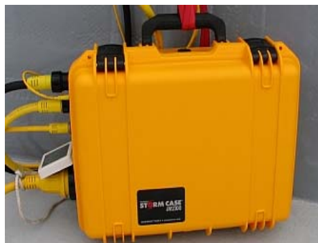
Figure 4 UnderwaySV power supply with all cables attached.
