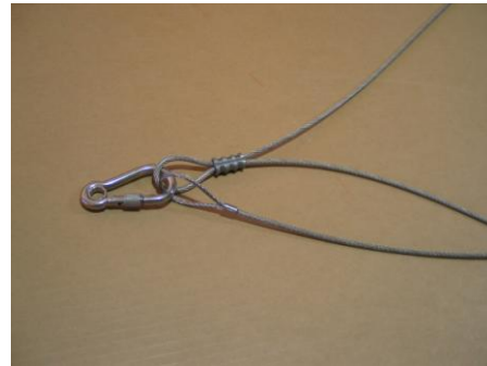
(Fig. 4.5) Safety cable, wire rope bridle, and carabiner ready for tow line
