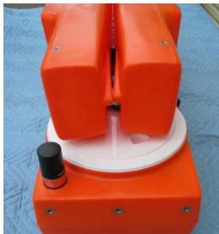
(Fig. 5.3) Correct arrangement of the hulls inside the Soft Case
