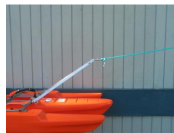
(Fig. 4.13) Negative towing angle. May submerge the boat, causing severe drag and possible loss of the boat
