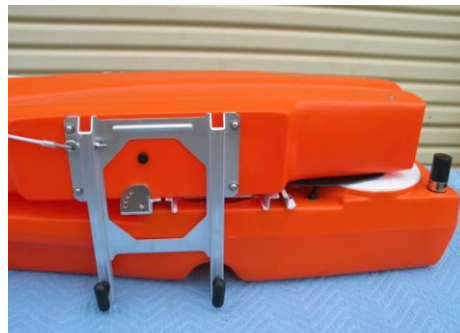
(Fig. 5.2) Nest the outriggers inside the Rigid Bridle flanges
