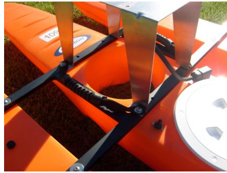
(Fig. 7.2) Place strap handle grommets over mount feet and attach
