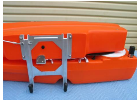
(Fig. 5.6) Nest the outriggers inside the Rigid Bridle flanges
