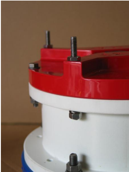
(Fig. 4.1) Mounting studs installed
