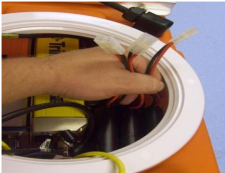
(Fig. 4.26) Position three 12 volt battery packs
