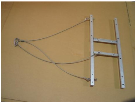
(Fig. 4.6) Wire Rope Bridle and Instrument Safety Cable attached to the Standard Crossbar
