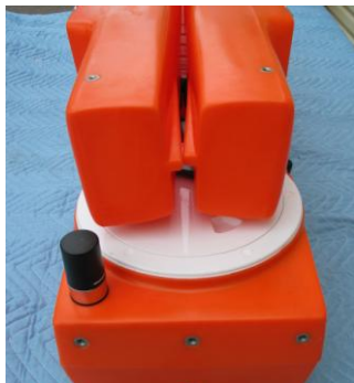
(Fig. 5.7) Correct arrangement of the hulls inside the ATA Case
