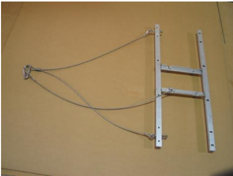
(Fig. 4.4) Standard crossbar with wire rope bridle and instrument safety cable
