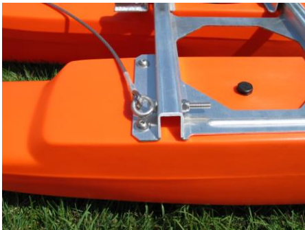
(Fig. 4.8) Wire Rope Harness eyebolt with lock nut installed on outrigger
