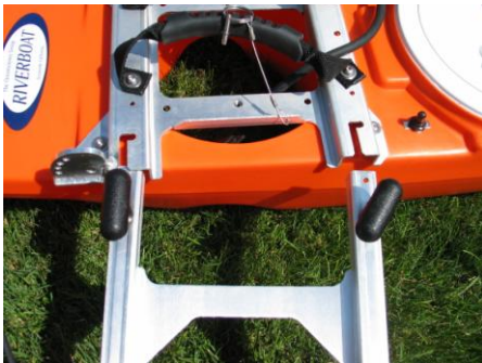
(Fig. 4.10) Insert the outrigger crossbar parts into the main hull, align, install the retaining pins, and tighten the thumb turns
