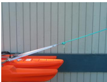
(Fig. 4.11) Preferred towing angle. Tether and bridle are collinear.
