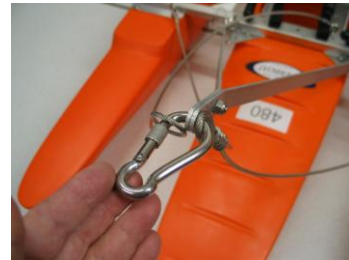
(Fig. 4.16) Carabiner with wire rope harness and instrument safety cable, attached to the Rigid Bridge
