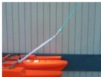
(Fig. 4.12) Positive towing angle. Acceptable
