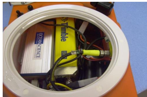
(Fig. 4.29) Position all cables and wiring away from the Oyster Heat Sink
