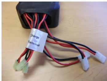
(Fig. 4.10) Tamiya connectors and identifying labels.
