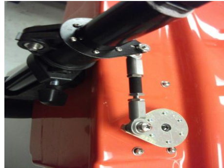
(Fig. 4.2) Position outdrive shaft so top of cable is 2-3" above outdrive steering arm
