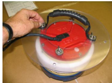
(Fig. 7.12) Carabiner with wire rope harness and instrument safety cable, attached to the Rigid Bridle
