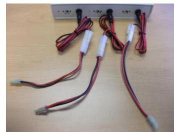
(Fig. 4.11) Connect three charging adapters to battery charger ports
