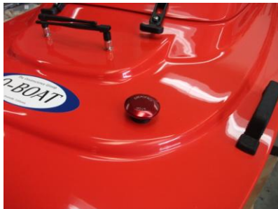
(Fig. 8.1) Q-Boat equipped with Emergency Stop button
