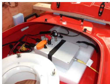
(Fig. 6.4) Insert VCU into foam tray and secure
