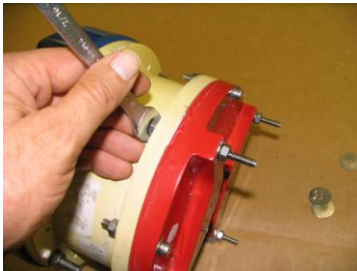
(Fig. 7.10) Install studs, nuts and flat washers on the ADCP
