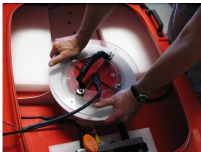
(Fig. 7.13) Press the instrument into the instrument well and align the screw holes
