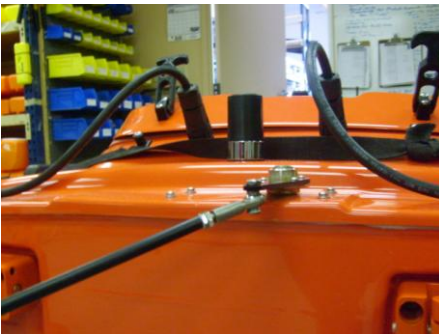
(Fig. 5.3) Connect short steering link to servo arm with screw
