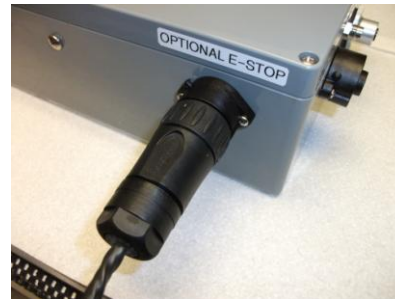
(Fig. 8.2) Emergency Stop cable connected to VCU
