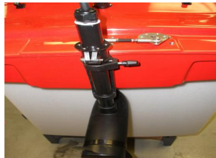
(Fig. 4.4) Connect motor power/control cable to the 4-pin bulkhead
