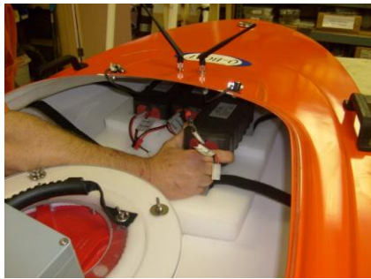
(Fig. 5.14) Load the battery packs in the hull with the leads facing toward electronics box
