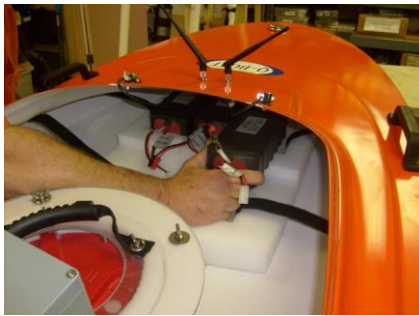
(Fig. 5.11) Load the battery(s) pack in the hull with the leads facing toward electronics box
