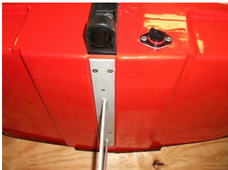
(Fig. 4.7) Properly installed skeg
