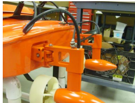
(Fig. 5.4) Connect short and long steering link to port outdrive with screw and washers
