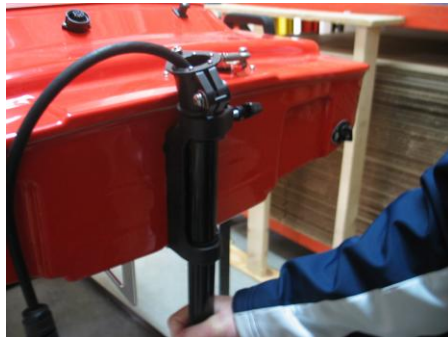
(Fig. 4.1) Insert connector and cable up through outdrive mount and steering
