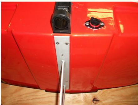
(Fig. 5.7) Properly installed skeg
