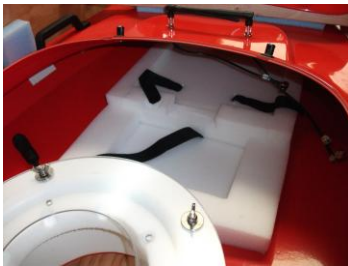
(Fig. 6.1) Foam tray for the VCU and battery(s)
