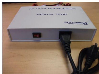
(Fig. 5.10) Connect the charger to the outlet and turn on front power switch to begin charge
