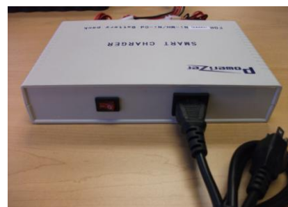
(Fig. 5.13) Connect the charger to the outlet and turn on front power switch to begin charge
