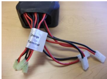
(Fig. 5.10) Tamiya connectors and identifying labels.
