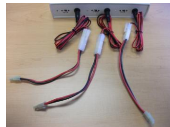
(Fig. 5.11) Connect three charging adapters to battery charger ports
