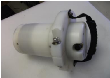
(Fig. 7.4) Install instrument clamp around S5 or M9 – Do not over tighten
