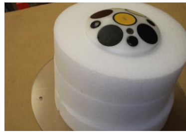
(Fig. 7.6) Place foam plug around the instrument
