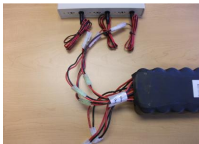
(Fig. 5.12) Connect greenish-yellow terminals to the adapters on the charger
