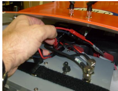
(Fig. 5.12) Connect the power leads to the electronics box
