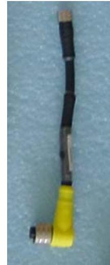
Figure 3. Depth sounder internal data connector cable.
