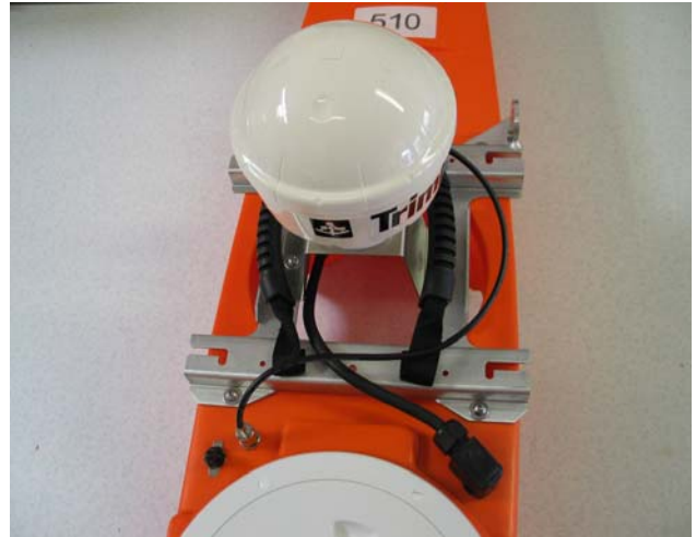
Figure 10. GPS dome antenna and antenna cable installed.
