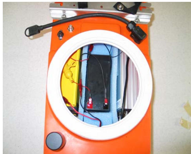
Figure 8. Equipment nested with foam spacers; power wires connected.
