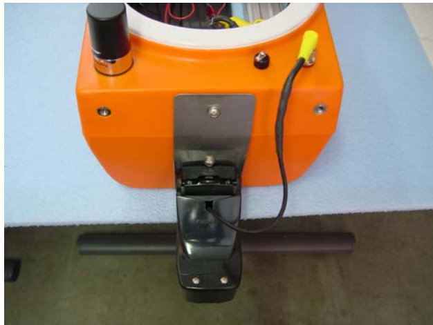
Figure 11. Depth sounder installed on Riverboat transom.
