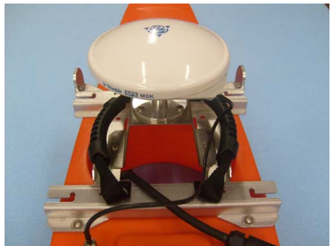
Figure 10. GPS dome antenna and antenna cable installed.
