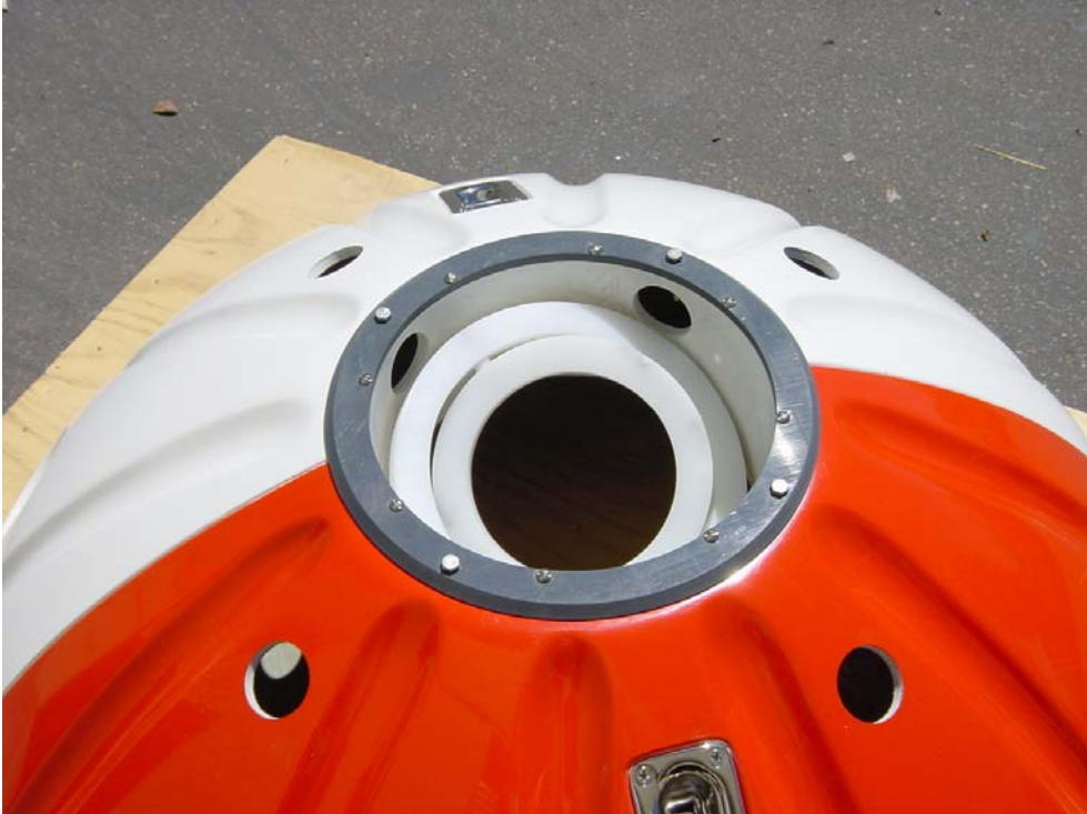
The Oceanscience Trawl Resistant Barnacle, with canister gimbal.
