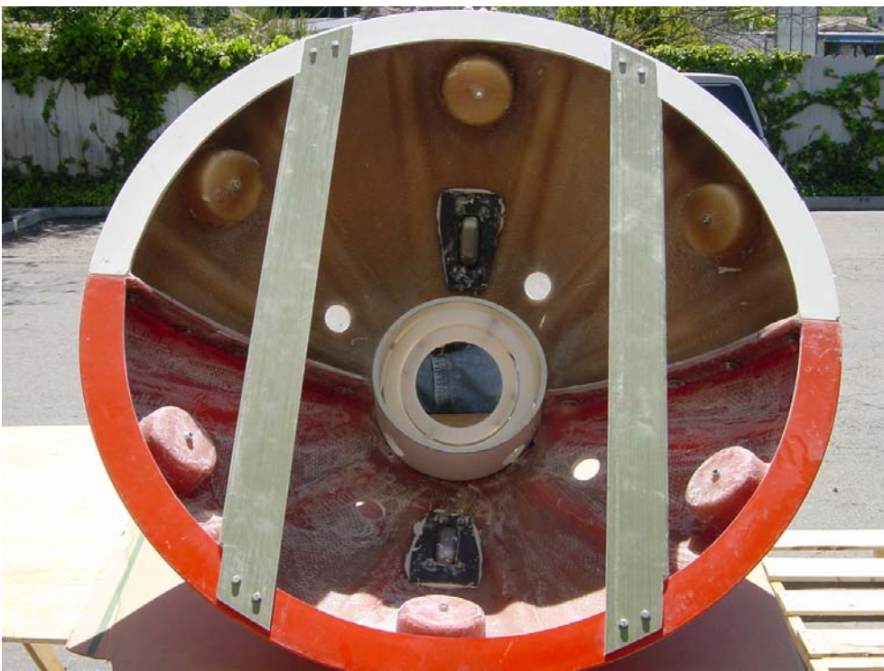
The Oceanscience Trawl Resistant Barnacle, with canister gimbal.
