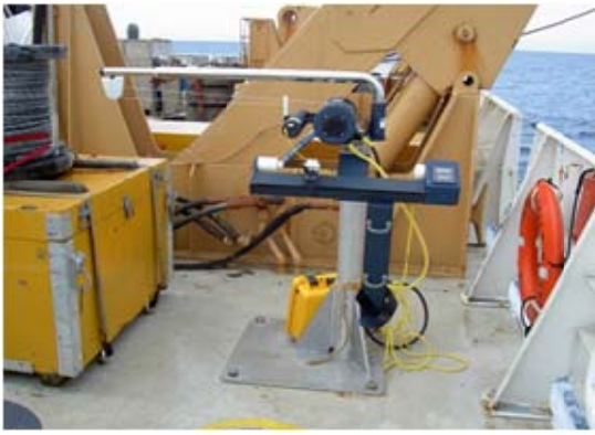
Figure 1. Series I UCTD Installed on R/V Ronald H. Brown.
